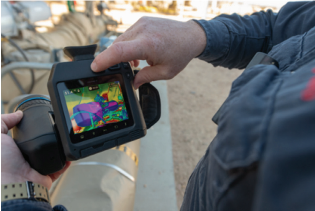
Images and videos from OGI devices such as the FLIR GF77 can provide a fact-base for troubleshooting safety and operations issues.
