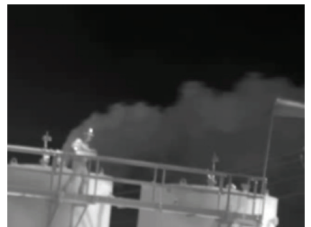
Example: Oil and gas industry worker on tank catwalk and inside gas leak from open thief hatch.
