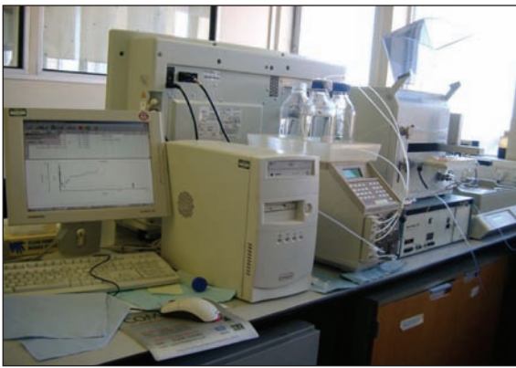
Figure 1 shows the HPLC system used for analysis consists of a pump, a detector, a fraction collector, assisted with a Gilson software.
