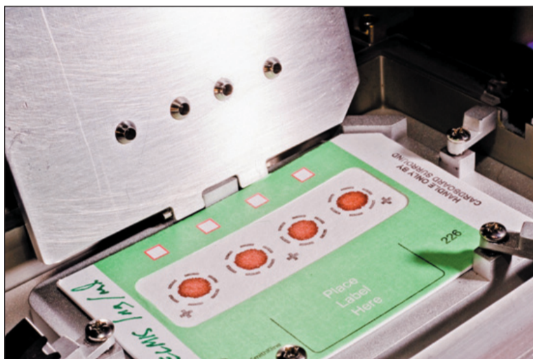
Figure 3. Photograph of a DBS card containing applied spots of whole blood. In this version stainless steel ferrules are employed to form the boundary region on the DBS card when the cover is clamped closed.
