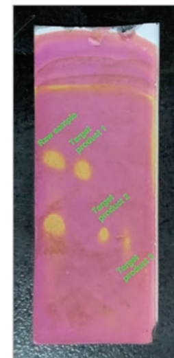
Figure 6. The Flash chromatogram of the sample by quaternary solvent gradient.
