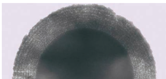
Figure 1: Schematic diagram of a Kinetex 2.6µm core-shell particle (a) and TEM micrograph of a cross-section through a Kinetex 2.6µm core-shell particle (b).
