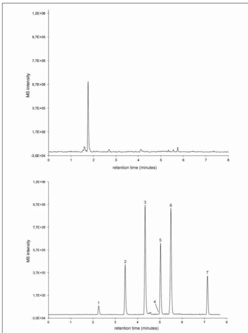
Figure 4. LC-MS base peak chromatogram (BPC) of seven pesticides spiked in porcine kidney and separated on a Chromolith® CapRod® RP-18 endcapped 150-0.1mm monolithic silica capillary column ( $m/z$  200-290). Top: Blank sample (undiluted), bottom: spiked sample (diluted 1:100). Mobile phase A: water + 0.1% formic acid, mobile phase B: acetonitrile + 0.1% formic acid; gradient: 20% B to 80% B in 10 min. For peak annotations see Table 1.
