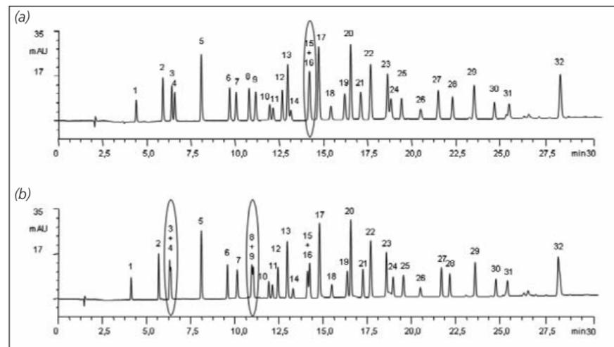
Figure 2. LC-UV chromatogram of a mixture of 32 pesticides separated on Chromolith® HighResolution RP-18 endcapped 100-4.6mm. Mobile phase A: ACN, B: 10mM NH<sub>4</sub>COOH, gradient: 10% A to 75% A in 30 min. Flow rate: 1mL/min. Detection: UV 254nm. Temperature: 35°C. Injection volume: 0.1µL.
