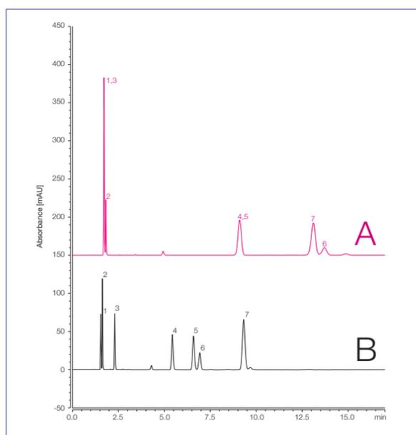
Figure 10: Separation of a test mixture on NUCLEOSHELL® RP 18plus and NUCLEOSHELL® Biphenyl
