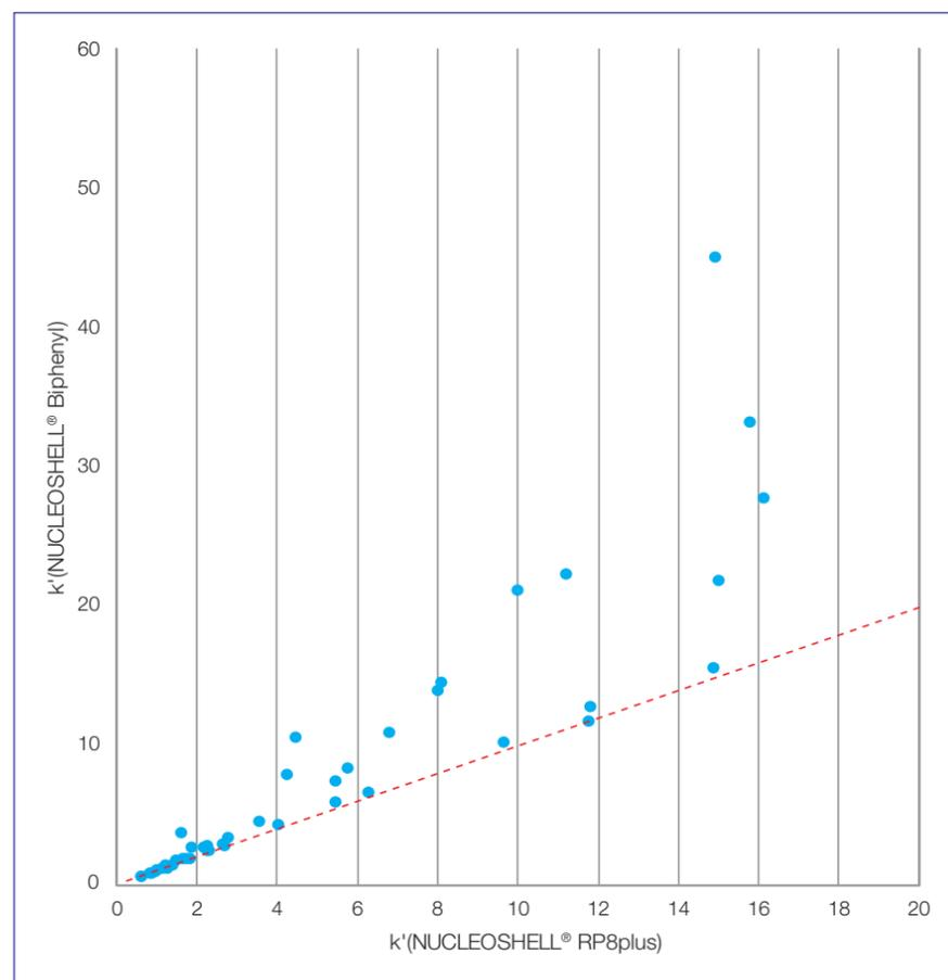
Figure 5. Comparison of NUCLEOSHELL® RP 8plus and NUCLEOSHELL® Biphenyl (acetonitrile/water)
