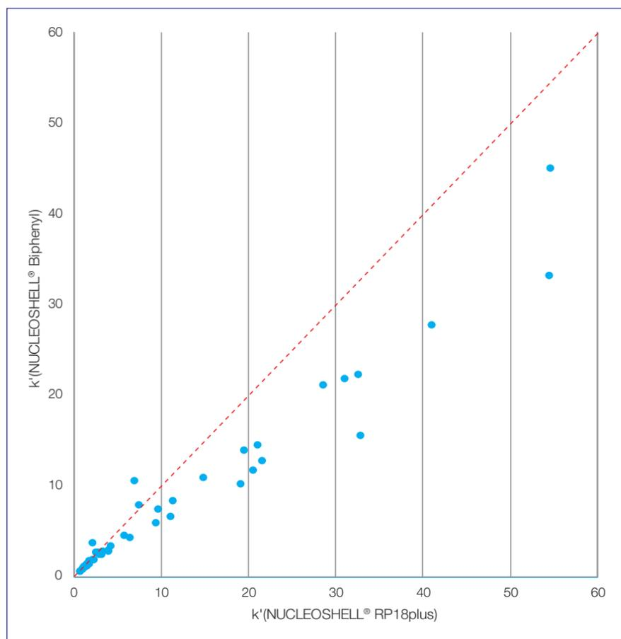
Figure 4. Comparison of NUCLEOSHELL® RP 18plus and NUCLEOSHELL® Biphenyl (acetonitrile/water).
