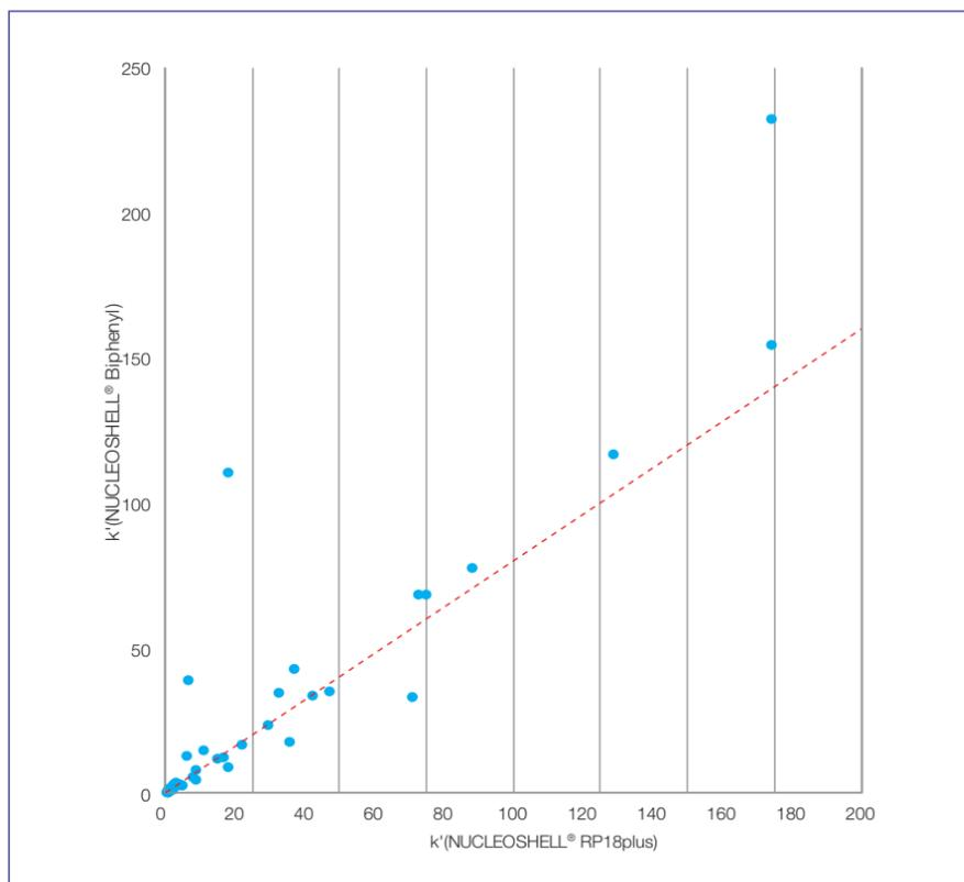
Figure 7. Comparison of NUCLEOSHELL® RP 18plus and NUCLEOSHELL® Biphenyl (methanol/water)
