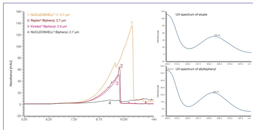
Figure 2. pH stability of different biphenyl sorbents using acidic gradients
