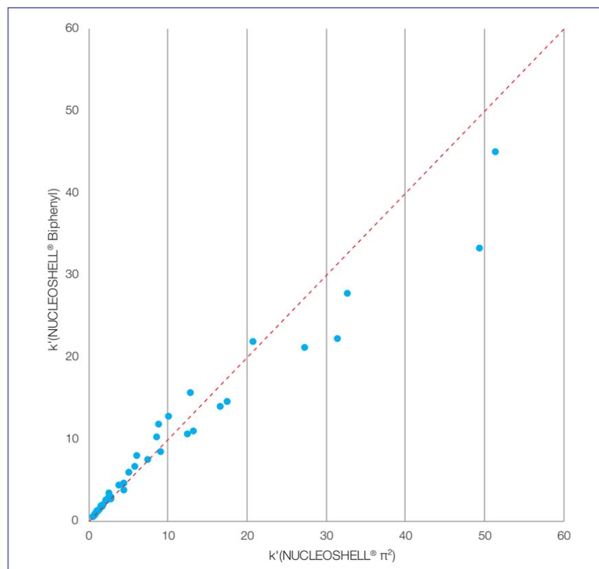
Figure 3. Comparison of NUCLEOSHELL®  $\pi^2$  and NUCLEOSHELL® Biphenyl (acetonitrile/water).
