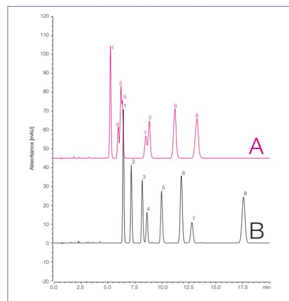
Figure 11: Separation of a test mixture on NUCLEOSHELL® π² and NUCLEOSHELL® Biphenyl
