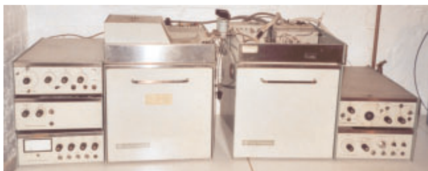
Fig. 3. A pair of Pyes!. The Pye 104 GC on the right was obtained from Dr Derek Stevenson of the University of Surrey whilst the (almost identical looking to the non-enthusiast!) Pye 105 on the left (the prep. version of the 104 was found by Dr Mark Powell (at the time of donation of Liverpool John Moores University).
