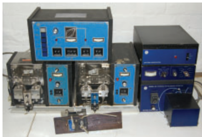
Fig. 4. A Waters HPLC system comprised of two M6000 A Pumps, the Model 660 gradient controller, a UV detector, and a U6K injector (lying on its side in front of the pumps). I'm not sure that the UV detector is quite right for this particular model, and I've been told that the "Rolls Royce" system came in a custom built cabinet (presumably with a proper mounting for the U6K). The 660 controlled the pumps via a pair of cables of which I have one. So anyone who can help with a contemporary UV detector, cabinet or controller cable.... I'd love to hear from you. I do have an authentic Waters refractive index detector which does fit with this set up.
