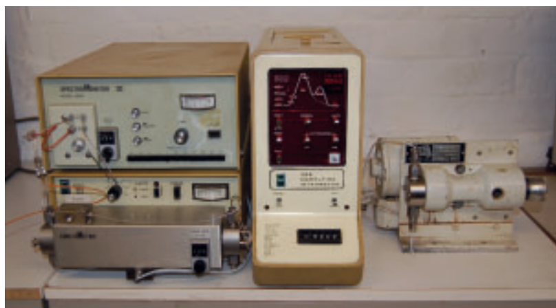
Fig 5. An old Milton Roy HPLC pump (on the right) from Klaus Borner together with a ex ICI/Zeneca Constametric III HPLC pump and UV detector. The upright device between the Constametric and Milton Roy pumps is a primitive a computing integrator. No peaks, just a roll of paper giving retention times and peak areas. Things HAVE got better.
