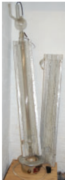
Fig 1. The all glass chromatograph from Gas Chromatography Ltd, circa 1960. This is very difficult to photograph because it's 1.4 meters high but only a few cm wide. The device is shown with the boiler pipe insulation that surrounded the whole thing opened up to show the 1.3m long "U" shaped, fixed, glass columns contained within the outer glass tube that acted as the oven.
