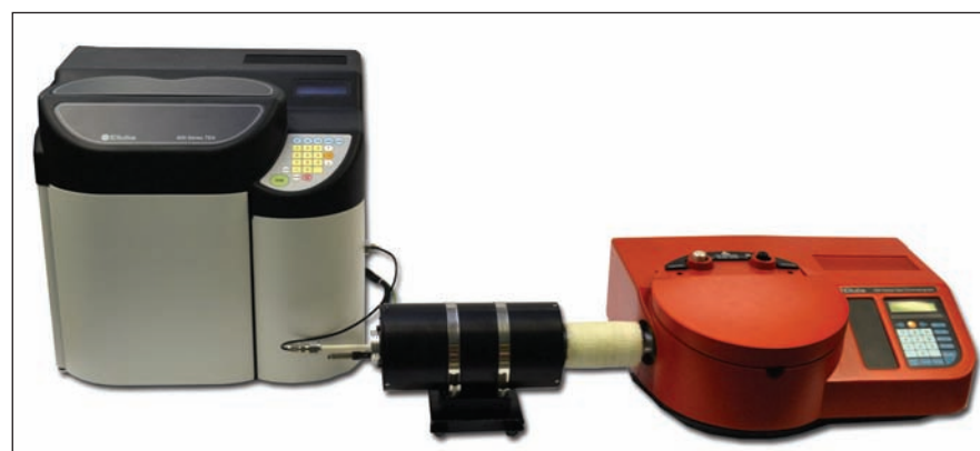
Figure 2. Thermal Energy Analyser (TEA) connected to a Gas Chromatograph (GC)
