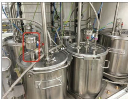
Figure 4: Fraction collection containers located inside a dedicated fume hood. The solvent level sensor (highlighted) is fitted to each container to prevent overfilling.
