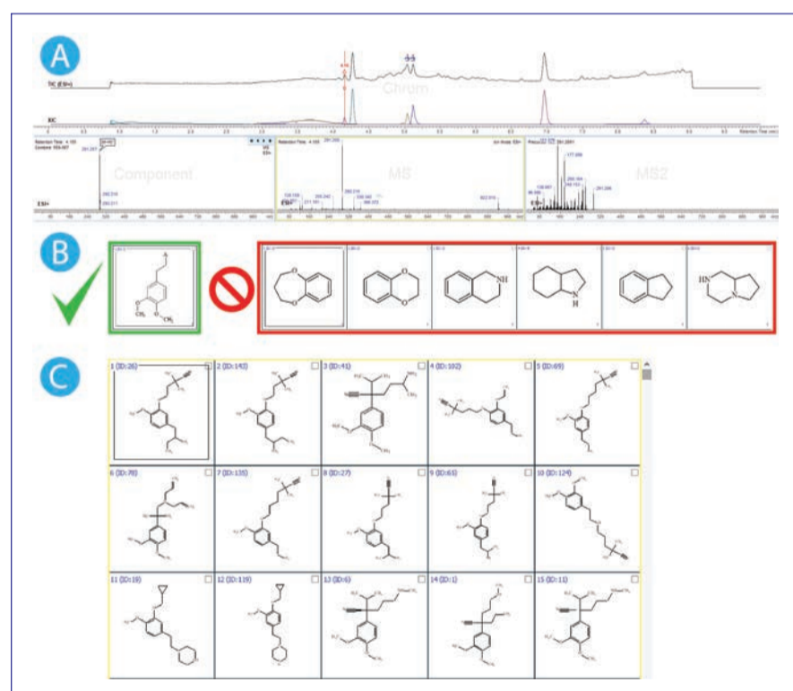
Figure 3. Depicting how the list of potential structure candidates for the component at RT = 4.155 min was reduced from 33,214 to 154 by filtering via a structure include/exclude list. A) The chromatographic and MS traces of the component at RT = 4.155 min, B) the applied structure include (dimethoxybenzene—green) and exclude (bicyclic substructures—red) lists, C) a subset of the resulting structure candidates for the component at RT = 4.155 min.
