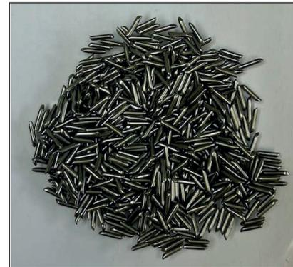
Figure 7: Stainless steel shot pins, unused.
