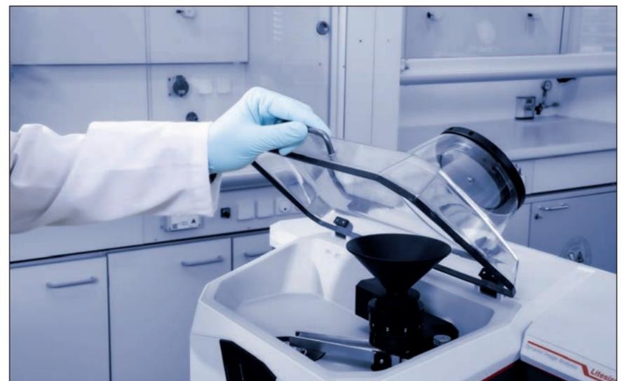
Figure 2: Safety hood on the Dry Jet dispersion unit mounted onto the Litesizer DIA 500.
